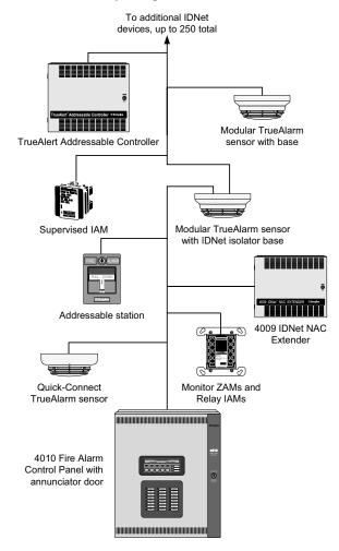
4010 Control Panel with Typical IDNet Devices
